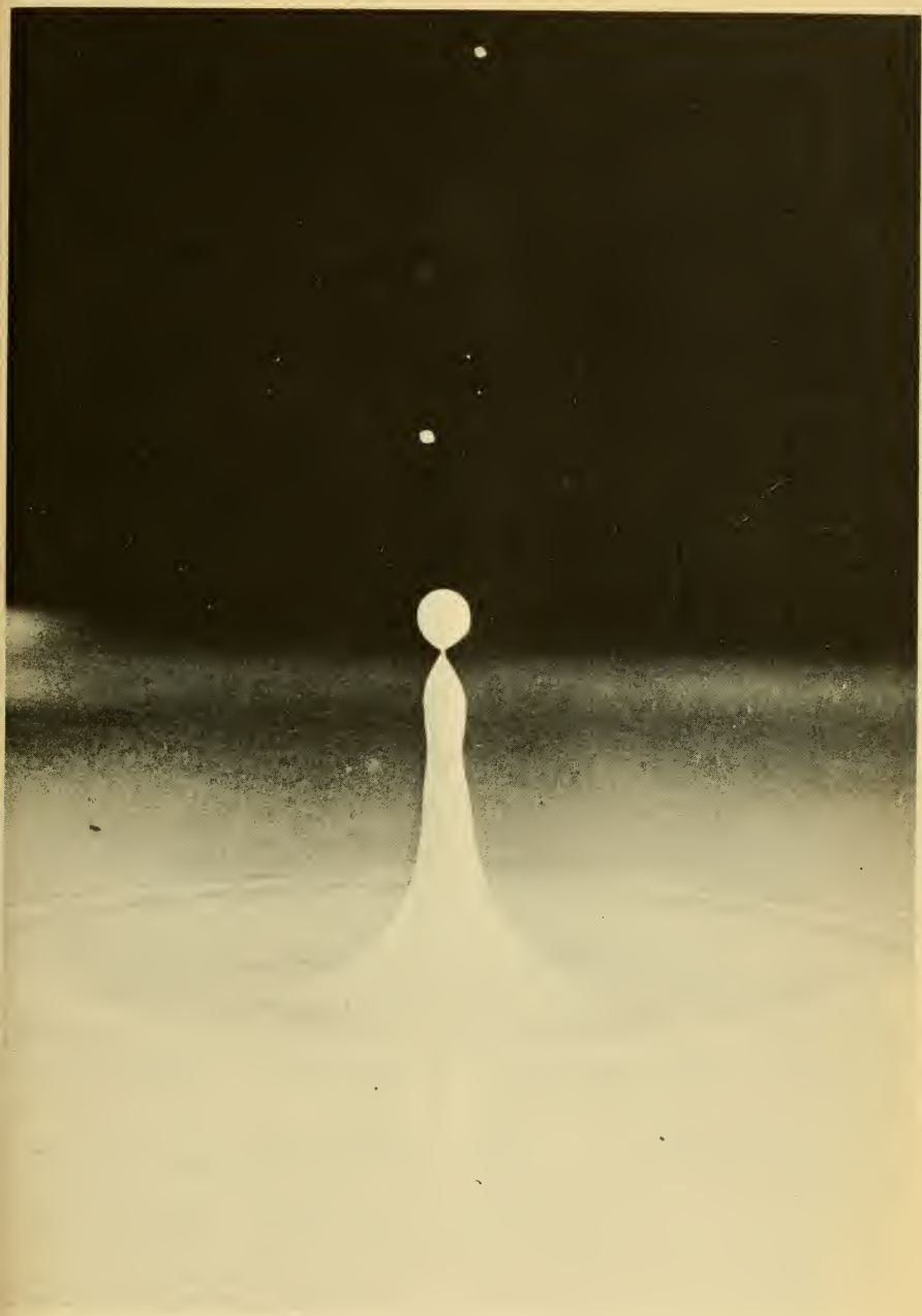
The latter phase of a splash: the crater has subsided, a columnar jet has risen up, and the jet is dividing into droplets. From Harold E. Edgerton, Massachusetts Institute of Technology
